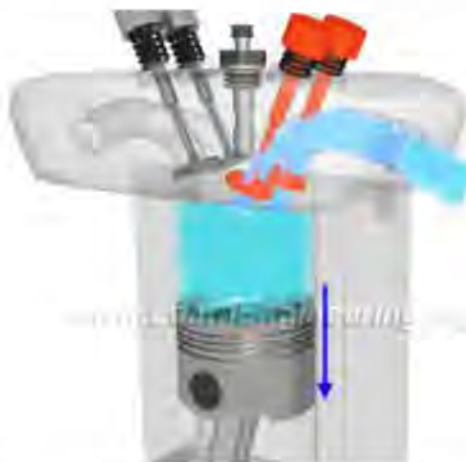
Figura 4.8. Admisia la motoarele Diesel (Sursa: Learn Engineering).
